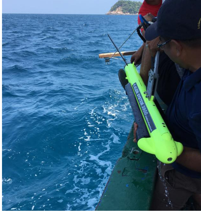
(Left) Dr. Tim Le Bas of NOCS inspecting the multibeam setup. The multibeam echosounder is mounted on the pole for the survey. (Right) Retrieving sidescan sonar at the end of the survey. | Photo by INOS
