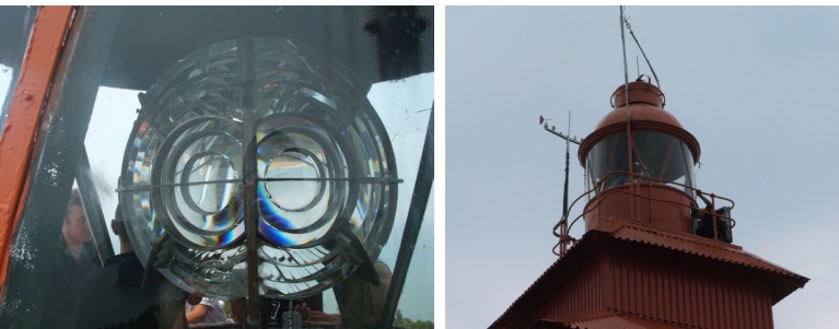
The old 'Stone-Chance lens' (left) at the Tanjung Po lighthouse in Kuching, Sarawak, and the lighthouse lantern (right).
